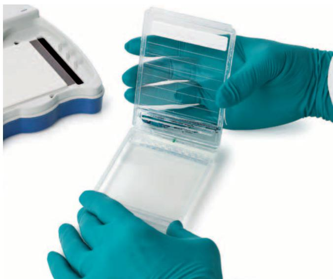
**Fig 2D.** The edge of the upper section of the cassette is used to remove excess gel in preparation for downstream processing.
