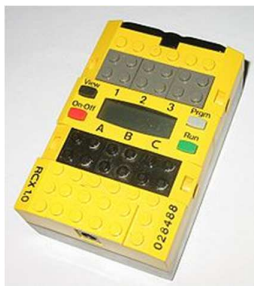
Figura 12. Bloc RCX. Figura extreta de: https://en.wikipedia.org/wiki/Lego_Mindstorms
